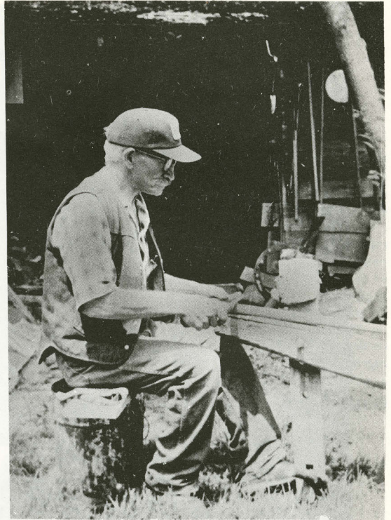
Gad, draw shaving a rung on the shave horse. His foot moves back and forth, tightening and loosening the rung as he shaves.
